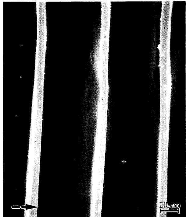
Fig. 24. The surface of radial wall of the tracheid after the moisture and heat treatments.
