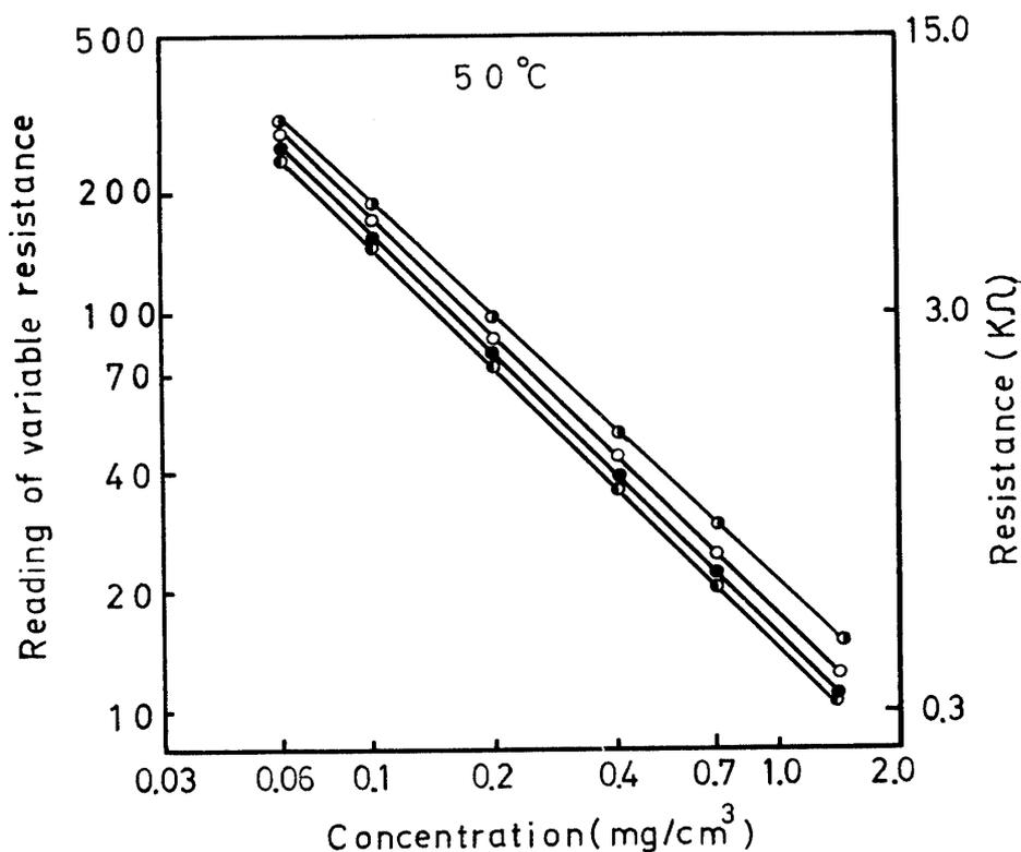
Fig. 1 An example of calibration curves for KCl
