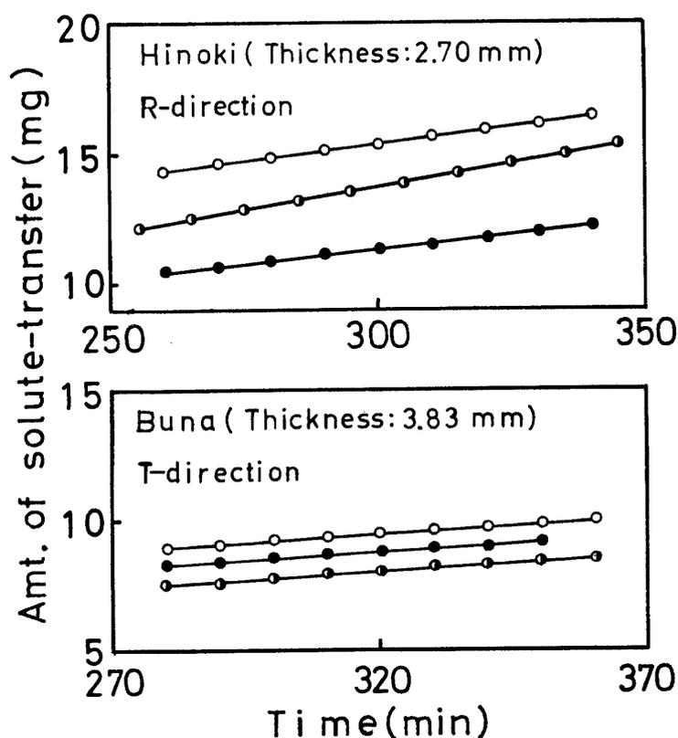
Fig. 4 Examples of diffusion curves of two-ply specimen for Hinoki and Buna woods
