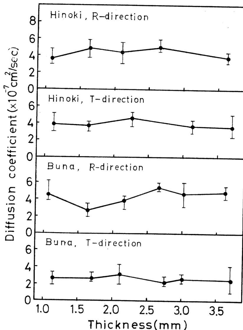
Fig. 3 Relationship between diffusion coefficient and thickness of test specimen for Hinoki and Buna woods
