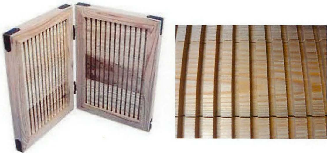
Fig. I-1 Slit material of Japanese cedar. [5]
