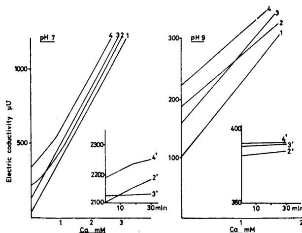
Fig. 5. Electric conductivity of casein solutions in the presence of various amounts of calcium at 15°C.
